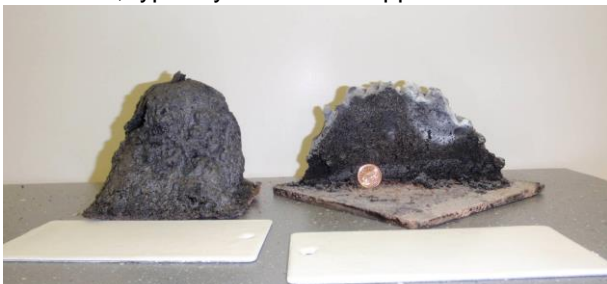
Metal coupons (TFI @ 60 mils DFT) before and after burning. Char insulates structural steel to provide a 2-1/2 hour fire rating per the testing indicated on page 2.
